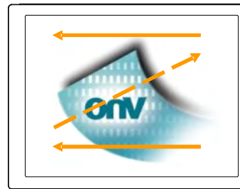
Fig. 2 Reverse scan (Pin19, RSV = High or VDD)
